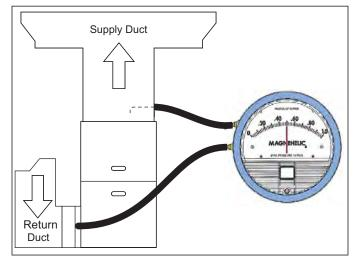
Set appropriate airflow per temperature rise for gas heating. Set appropriate airflow per "Blower Performance CFM" table for cooling/heat pump heating operating based on outdoor unit size and external static pressure.
